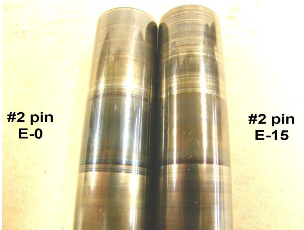
Figure 50: Cylinder 2 Wrist Pin Comparison, E0 on Left, E15 on Right
