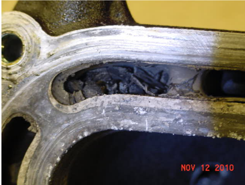
Figure 23: Mineral Deposits in Cooling Jacket, E0 Verado 1B812775A
