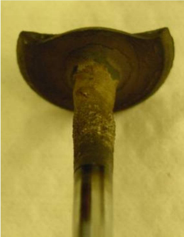
Figure 25: Broken Exhaust Valve from E15 Verado 1B812776, Top Valve in Cylinder 3
